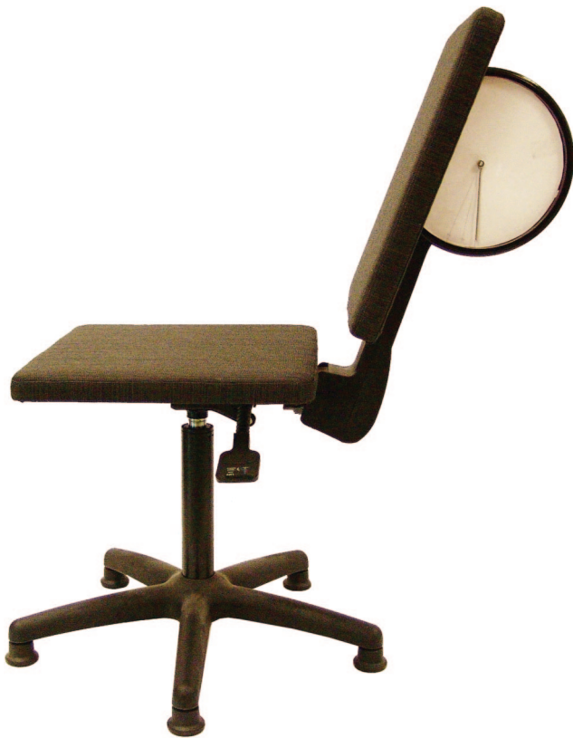
Figure 1. The custom-made experimental chair featuring adjustable seat pan and backrest with a gravity-dependent goniometer attached. Seat height was adjustable to ensure consistent hip and knee angulation across participants.
